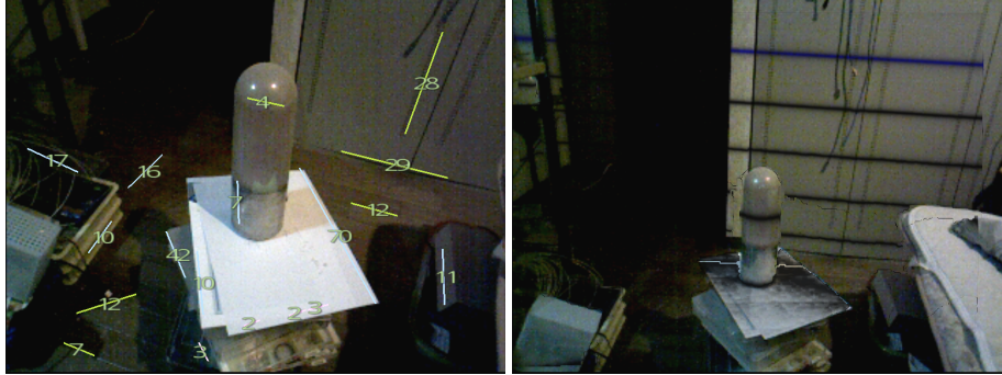
Fig. 6. Left: Length annotation cannot display height of the round-end cylinder Right: Height annotation reveals height of 1.5 units, which corresponds to 30 cm
