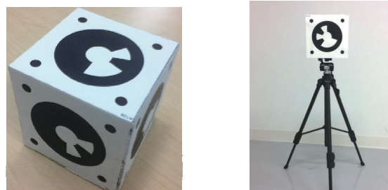
(a) Dice-shaped marker (radiation source)
