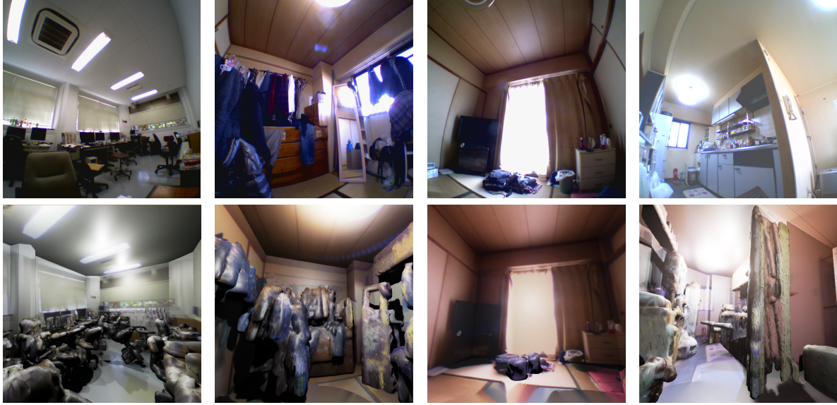
Figure 3.49: Top row: photos of each scene. Bottom row: reconstruction, rendered by the runtime subsystem. From left to right: un1 , re1 , re2 , and re3 .
