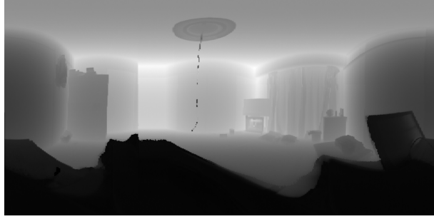
Figure 2.5: An example of distance image of a room. Brightness of each pixel is proportional to the distance between the camera and a point on a 3D surface pointed by the pixel.
